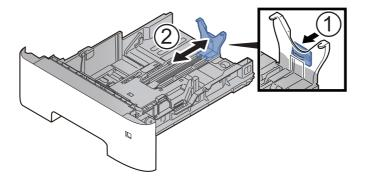
**3** Attach the auxiliary guide to the paper length guide as shown in the illustration.
